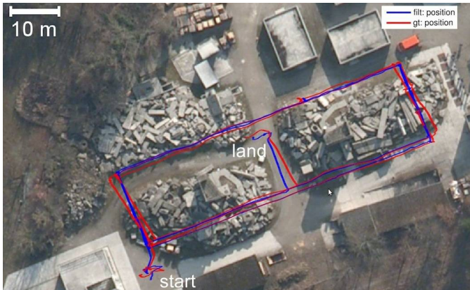
Fig. 13. After a short initialization phase at the start, vision-based navigation (blue) was switched on for successful completion of a more than 350 m-long trajectory until battery limitations necessitated landing. The comparison of the estimated trajectory with the GPS ground truth (red) indicates a very low position and yaw drift of the real-time onboard visual odometry.
