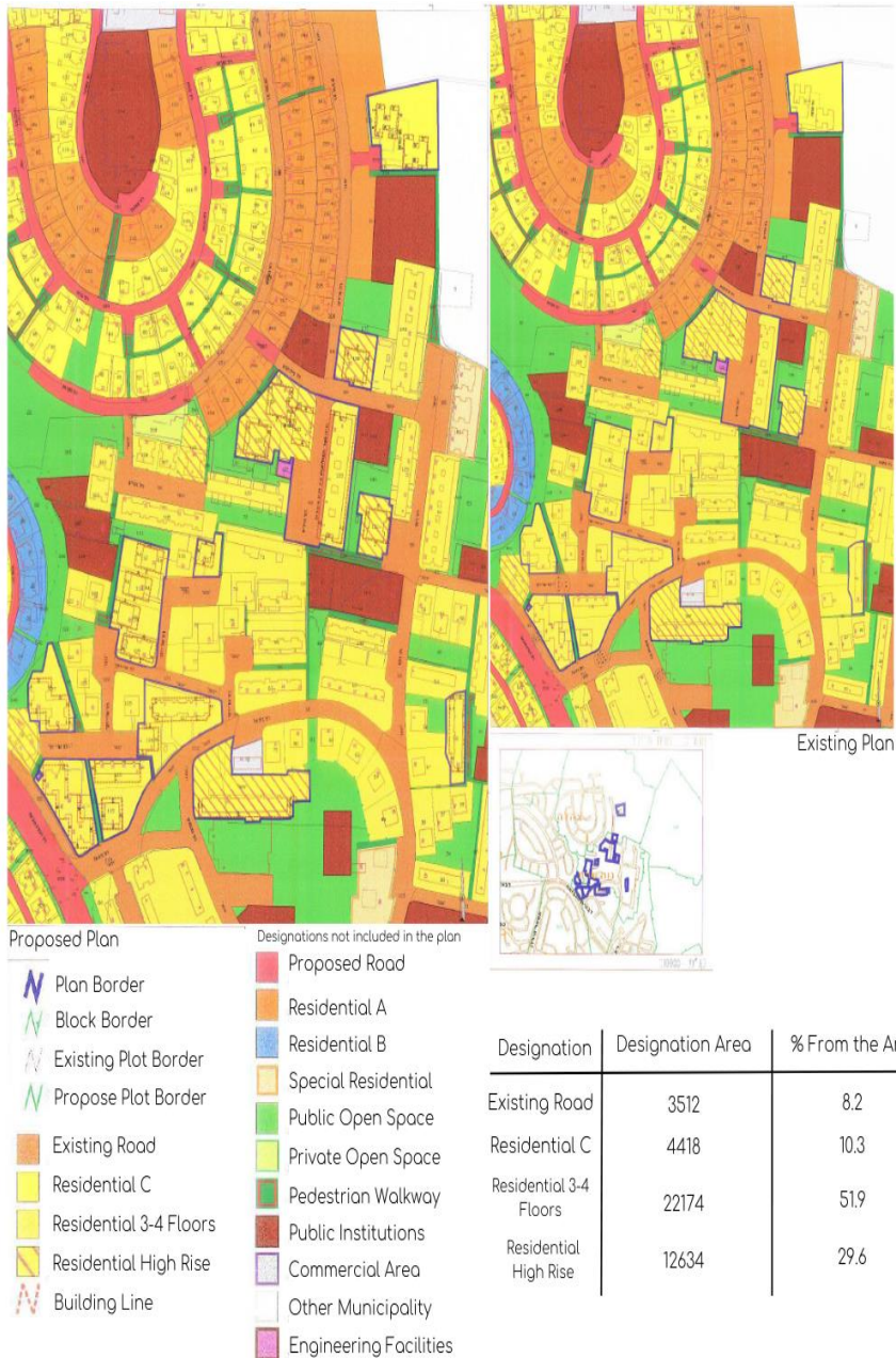
Map 3.7 - An example of a City Building Plan for the improvement of housing conditions and additional construction in a neighborhood in Tel Aviv. Source: (Planning Authority, 1999)
