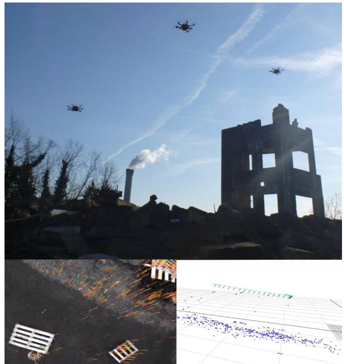
Fig. 14. SFLY helicopters during a demonstration of autonomous exploration at the firefighters training area in Zurich. (Bottom left) Feature tracks. (Bottom right) Online-built 3D sparse map used for local navigation.
