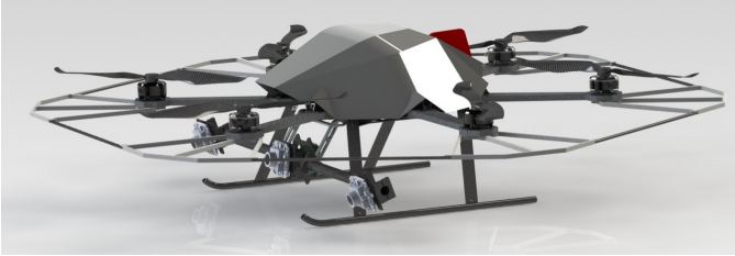
Fig. 5. Complete CAD model including three cameras on the SFLY hexacopter.
