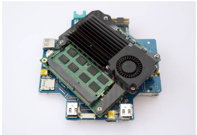
Fig. 3. On-board computer AscTec Mastermind featuring a Core 2 Duo CPU
