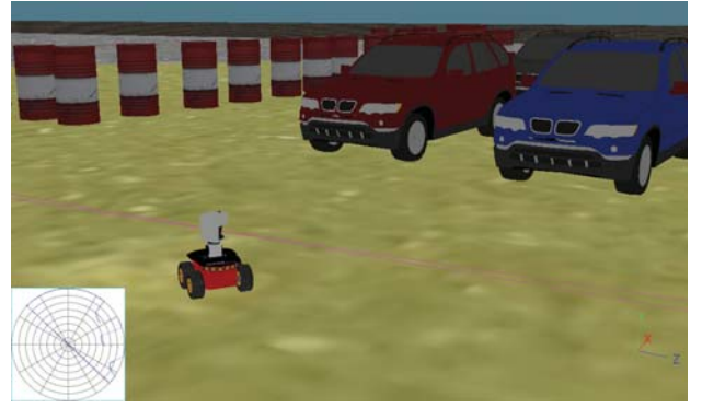
Fig. 3. The Open Dynamics Engine mobile robot simulation environment.
