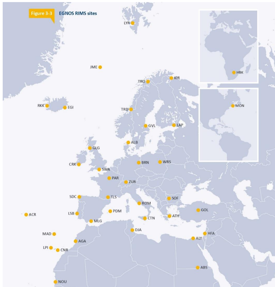
Εικόνα 6: EGNOS Ground Segment network of Ranging Integrity Monitoring Stations (RIMS)(Πηγή: https://gssc.esa.int/navipedia/index.php/EGNOS_Ground_Segment )
