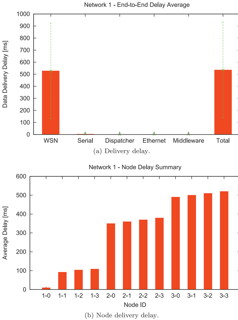
Fig. 17. Network 1 delivery delays. These are low and bounded, dominated by WSN delays.
