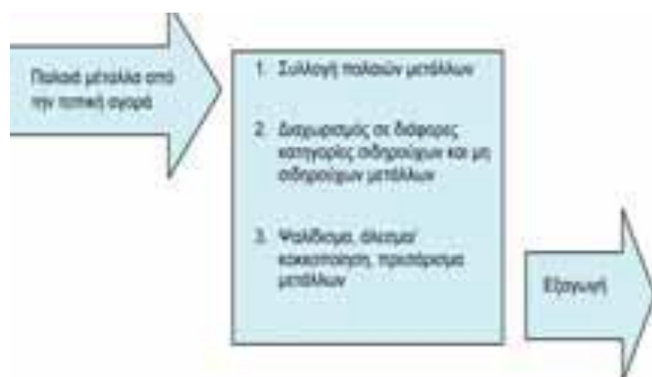
Figure 3.1: Process of scrap metal recovery
