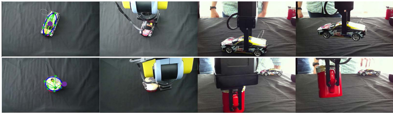
Fig. 5. The proposed method is capable of providing accurate grasping point estimations that enable the adequate manipulation of either a car or a cup. Here the fitted ellipse utilized through the manifold modeling process is shown with a blue line, while the purple dot is the grasping point computed.
