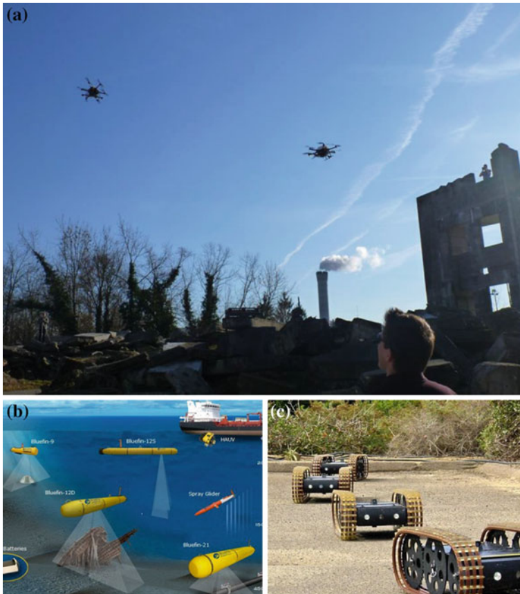
Fig. 10.1 Real life applications of teams of Autonomous Vehicles, operating under different environment, constructed under different design architectures. a Unmanned Aerial Vehicles ( UAVs ) in continuous infrastructure monitoring to prevent accidents [5]. b Autonomous Underwater Vehicles ( AUVs ) for underwater archeology and post-disaster infrastructure inspection. c Autonomous Ground Vehicles ( AGVs ) during ground surveillance task
